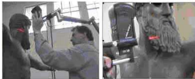
Figure 16 - Making the sweeping of the Zeus/Poseidon with a Scanner by Laser.
